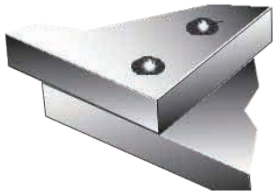
Plug Welds (Fig 1-19j)
